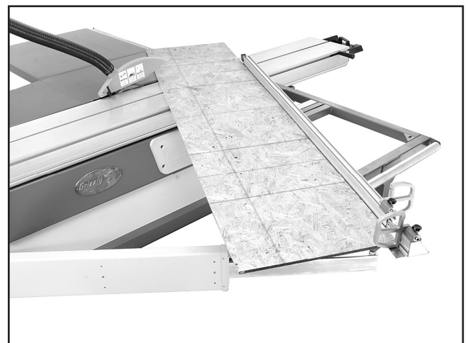
Figure 65. Example of miter cutting operation.
